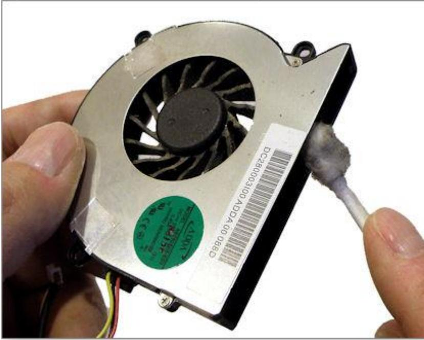
**a** 4. Clean the vents and heat exchanger the same way. As you see in Figure 6, a barely damp cloth works well.
