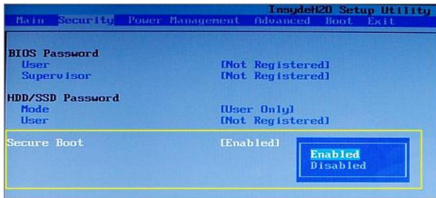
Figure 4. Secure Boot is typically enabled by default. Select Disabled to use a non-Microsoft rescue/repair disk.
