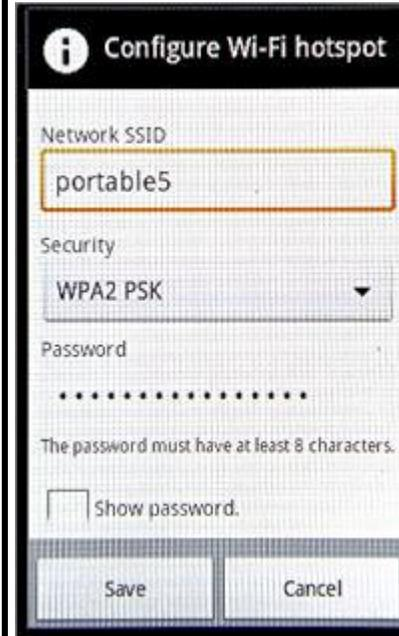
Figure 3. **Tethering/hotspotting** lets your smartphone act as a standard access point for any Wi-Fi-capable devices (such as Windows laptops).
